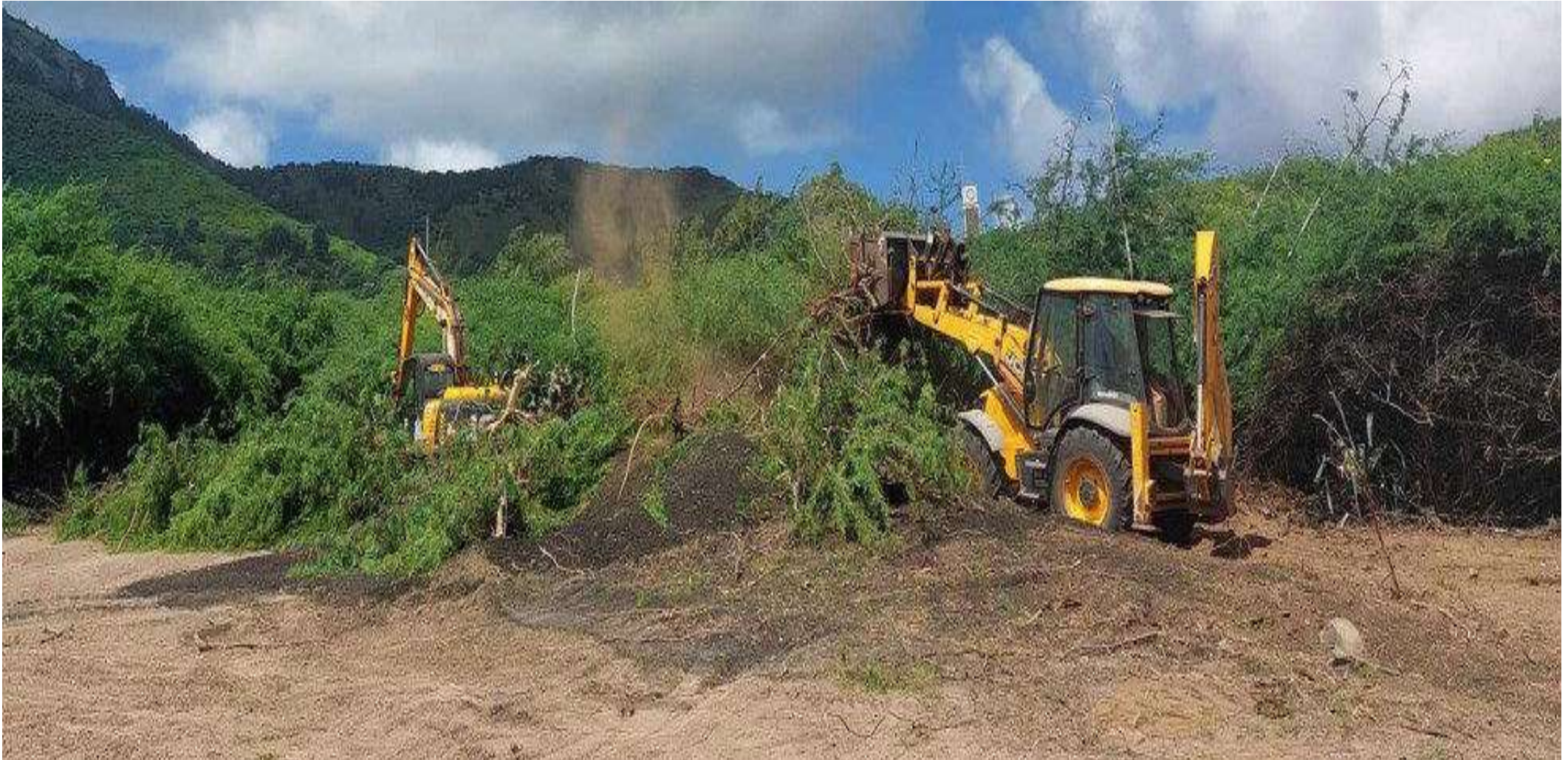
Figure 6: Machinery such as JCBs are used to remove Mexican thorn from road verges © L. Shearer
